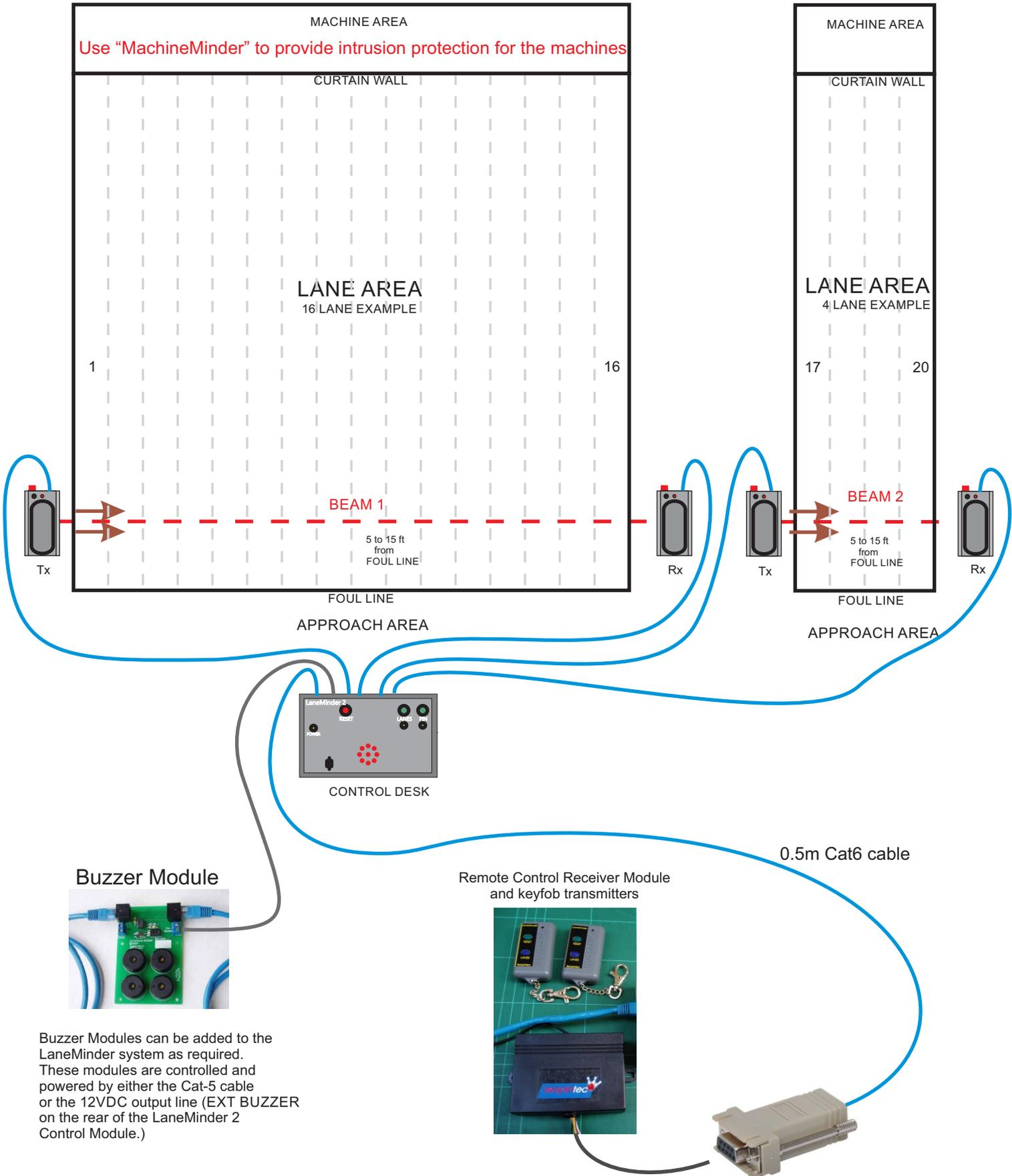
Buzzer Modules can be added to the LaneMinder system as required. These modules are controlled and powered by either the Cat-5 cable or the 12VDC output line (EXT BUZZER) on the rear of the LaneMinder 2 Control Module.)
